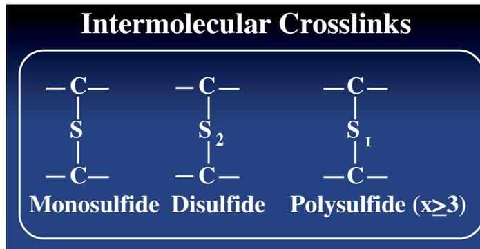
As one can see the carbon-carbon bond has a higher bond energy (350kJ) than the sulfur-carbon bond (285kJ) formed by the EV (Efficient Vulcanization) sulfur cure system and a much stronger bond strength than the sulfur-sulfur bond (< 270 kJ) formed by a CV (Conventional Vulcanization) sulfur cure system.
