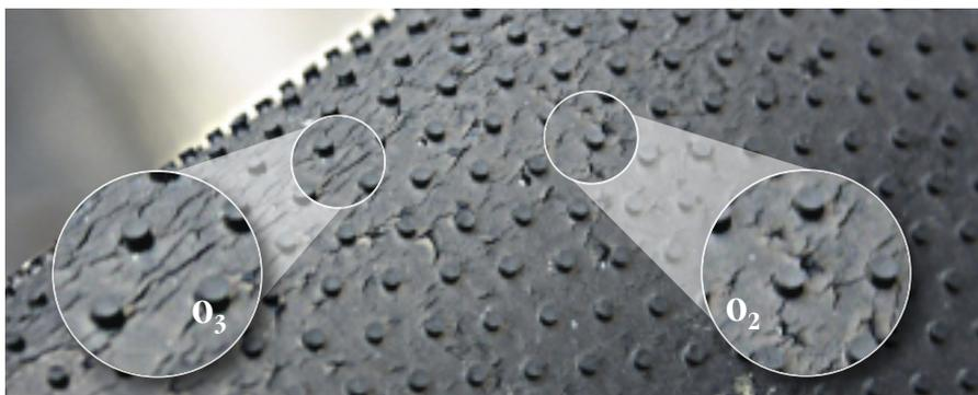
**Effect of  $O_3$  on unprotected rubber**      **Effect of  $O_2$  on unprotected rubber**
